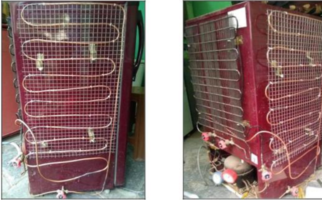
Fig:2.4 Refrigerator with Twisted taped Condenser
