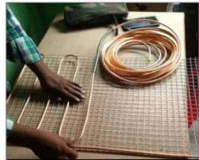
Fig: 2.3 Insertion of the twisted tape into the condenser coil
